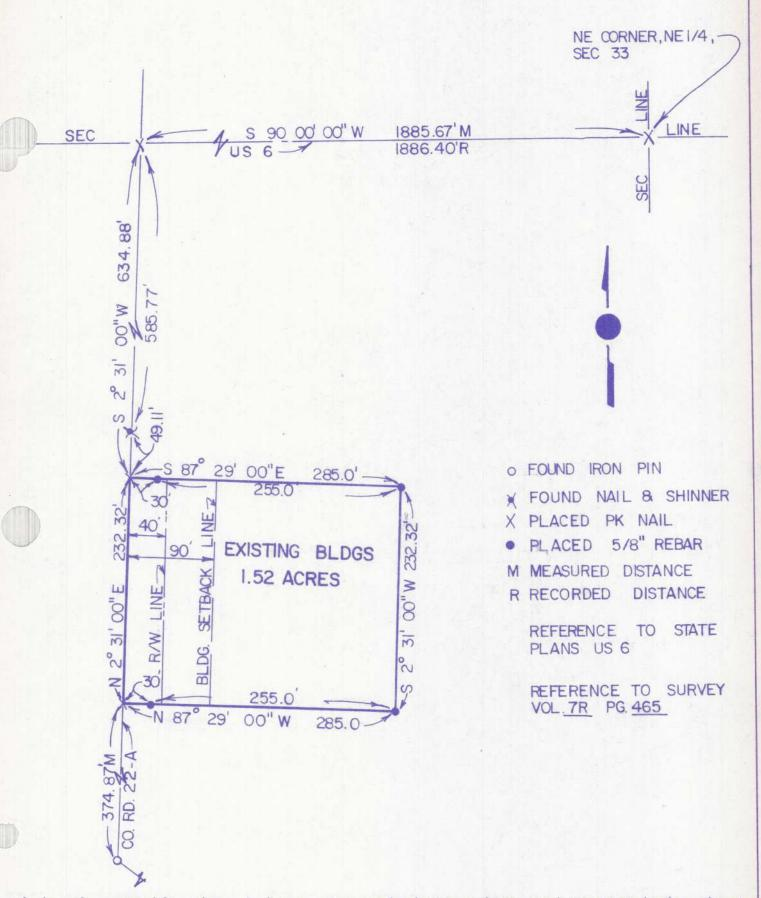
I hereby certify that I have surveyed the premises and prepared the above plat and that said plat is correct to the best of my knowledge and belief. I dimensions are shown in feet and decimal parts thereof. This survey has en recorded in Vol. 10R Page 106 of the Williams County Record of Surveys. ATE OF
